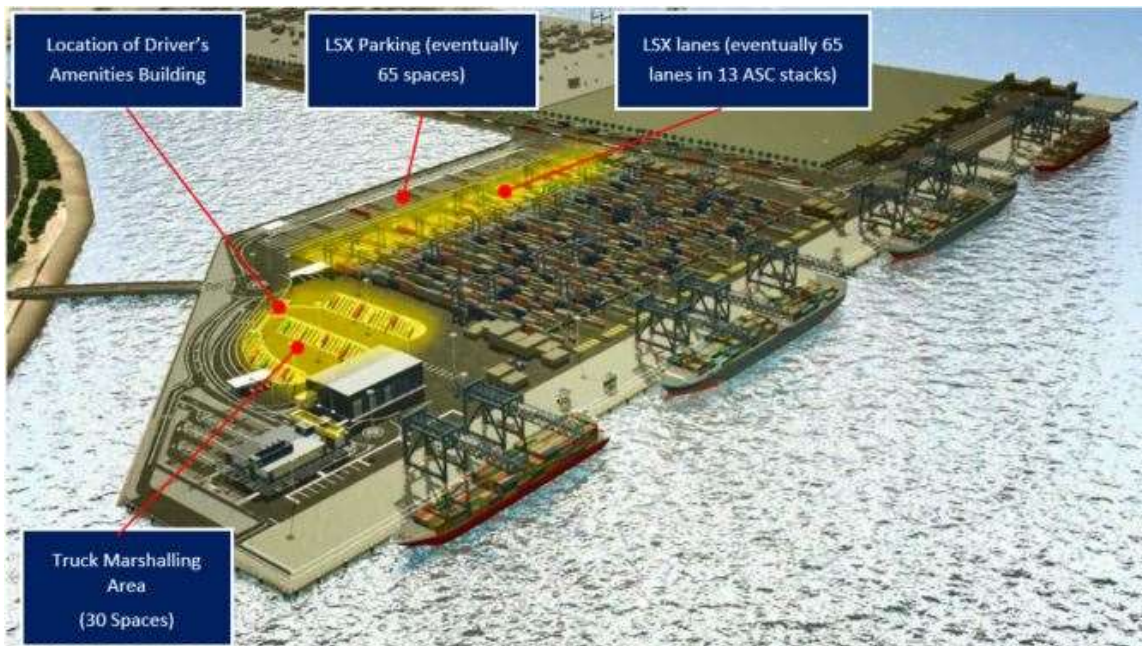
Figure 12 - Trucks Movement Area
