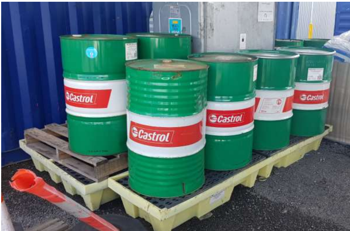
Photo 6: Drums on pallet bunds (note deviation from NSW EPA bunding requirements).
