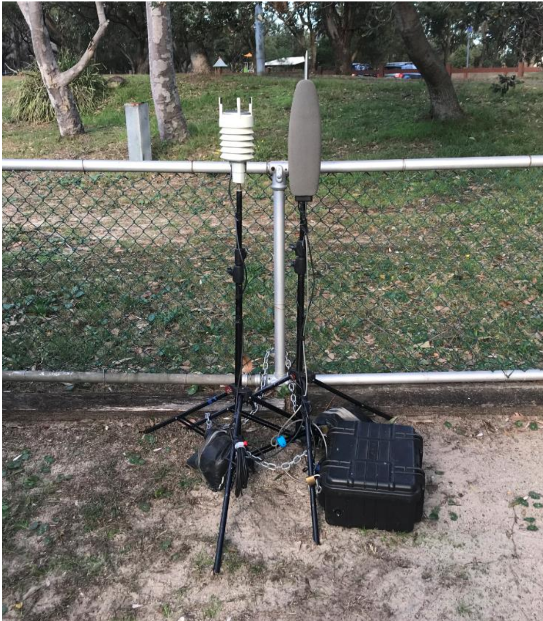
Figure B2: Noise logger and weather station installed at 34 Dent Street, Botany
