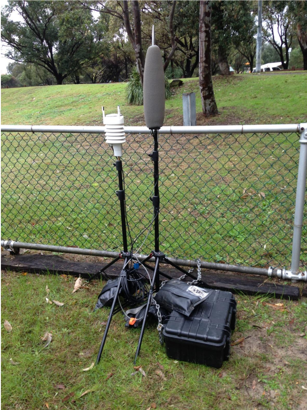
Figure B2: Noise logger and weather station installed at 34 Dent Street, Botany
