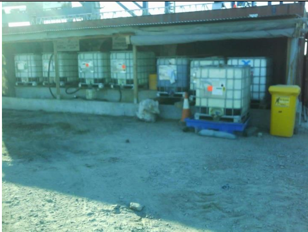
Photo: LOR1: Liscon IBC concrete additive and waste storage. One IBC outside covered area, no relevant labelling on waste IBCs
