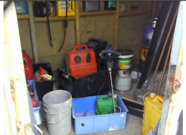
Photo GC2: Inside the storage cabinet. Whilst some fuels and chemicals are within tubs, some (including highly flammable thinners) are not
