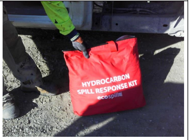
Photo LOR4 – CG Civil. Incorrect type of spill kit for type of substances used (paints used are water based, not hydrocarbon)
