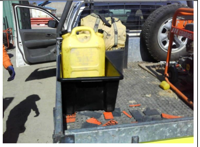
Photo LOR16 – Plastic tubs for transporting and storing minor quantities of fuel on site. Subcontractors required to comply. Spill kits carried on board
