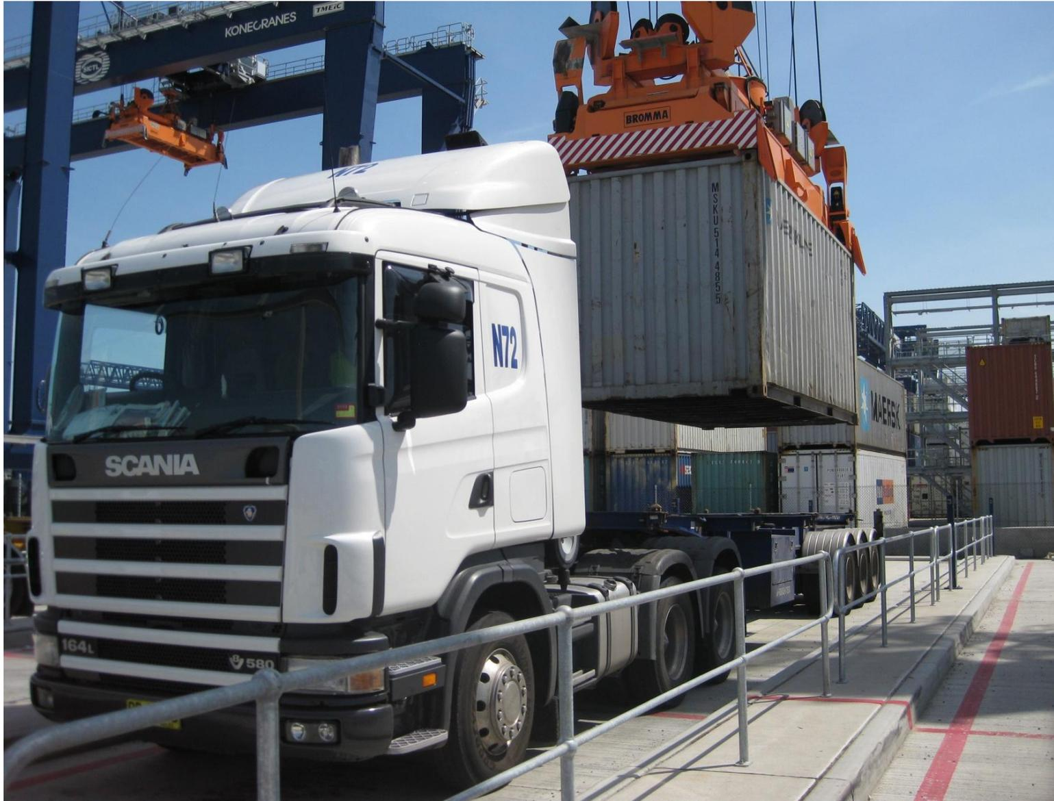
Figure 6: ASC unloading container
