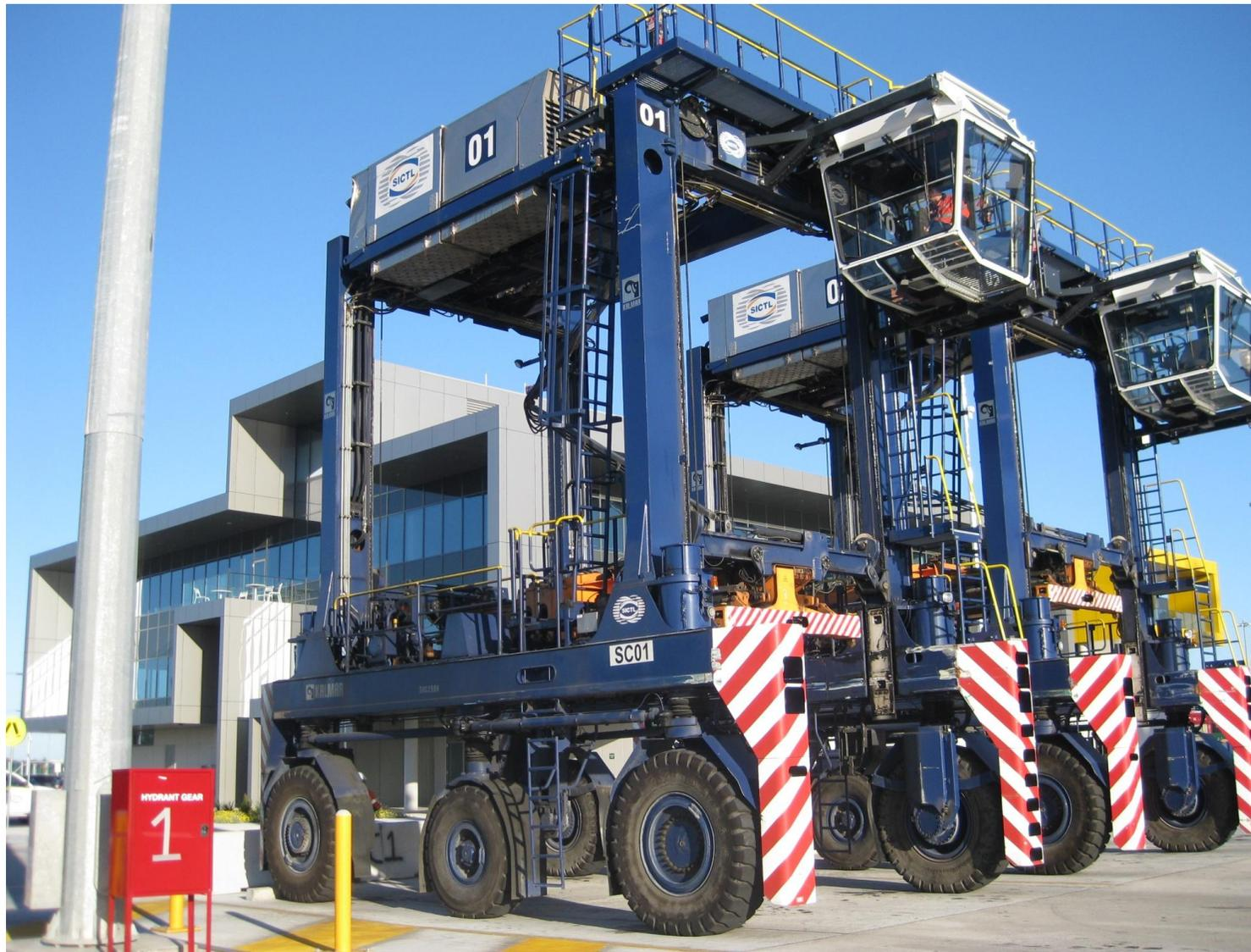
Figure 4: Shuttle Carrier
