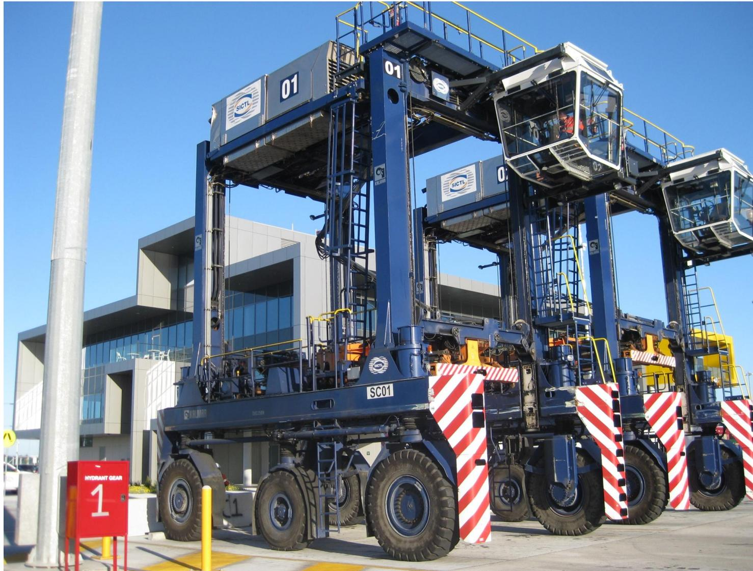
Figure 4: Shuttle Carrier
