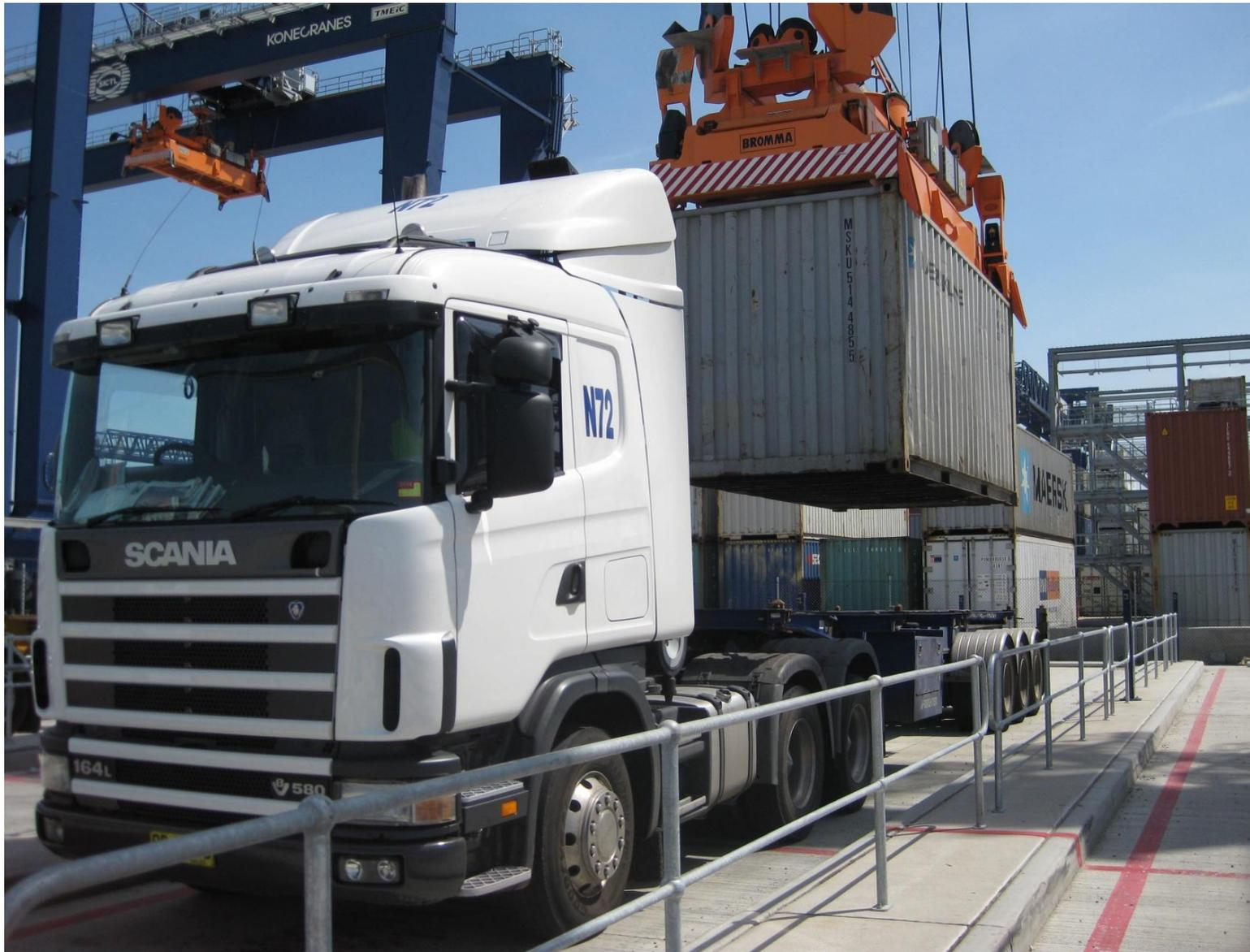
Figure 6: ASC unloading container
