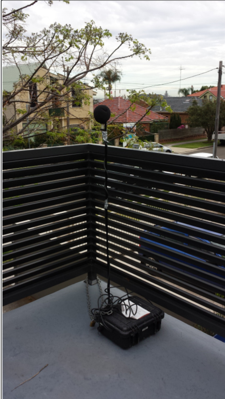
Figure B1: Noise logger installed at 59 Jennings St, Matraville
