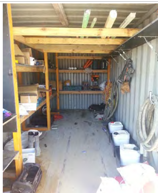
Photo004: KNF site container in an excellent state of housekeeping. Note the use of secondary spill containment (black plastic buckets). This level of care is taken all over site at Port Botany and not seen so predominantly on any other site I inspect. Well done for setting a high standard.
