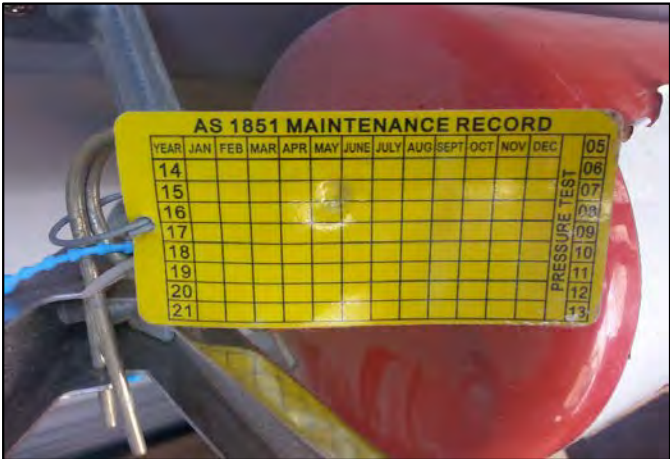
Photo 005: Example of one of the incorrectly stamped maintenance record. This record shows it was performed in
