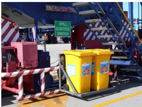
Spill Kits situated at the Quay Cranes.
