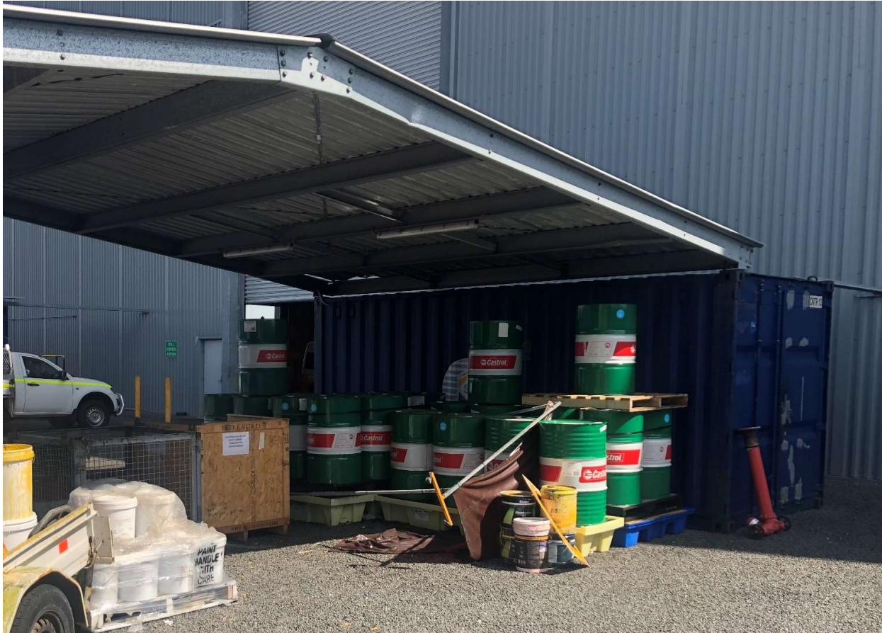
Plate 8: Over stacking of drums on spill pallet near workshop
