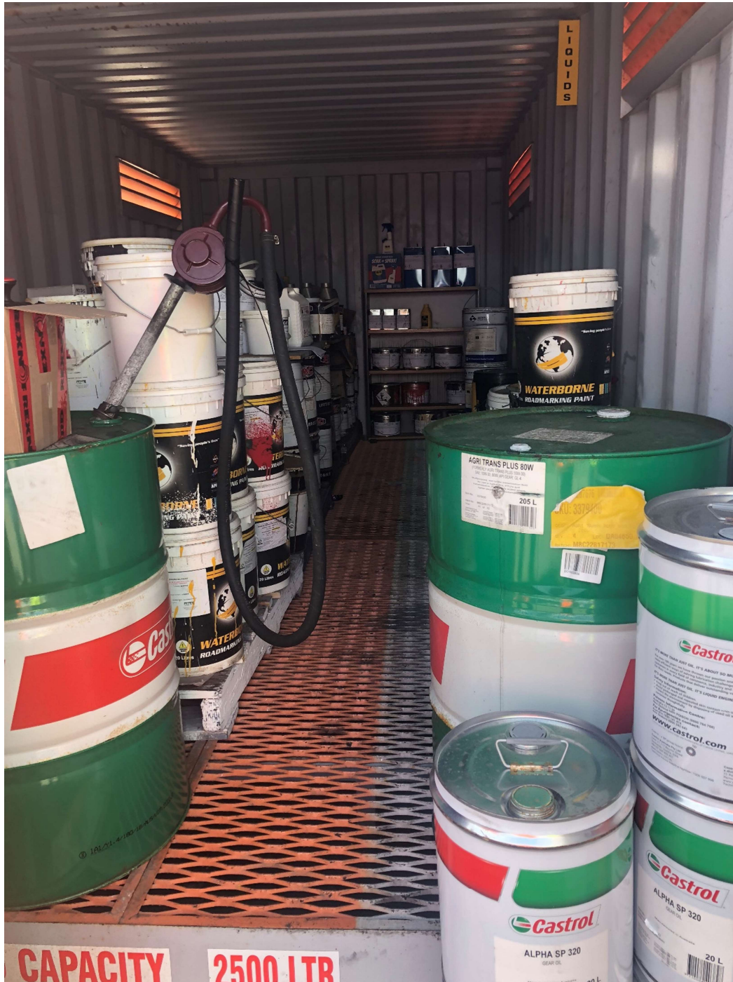
Plate 1: Paint containers, batteries & other liquids stored in bunded container
