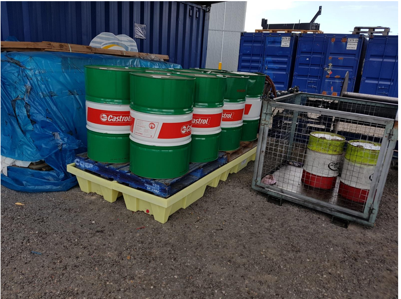
Plate 10: Overstacking of drums on spill pallet
