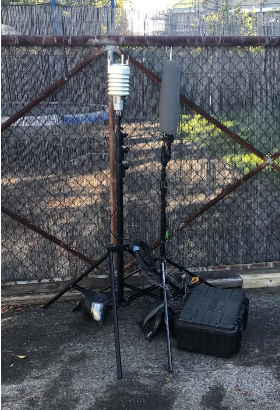
Figure B2: Noise logger and weather station installed at 11 Dent Street, Botany
