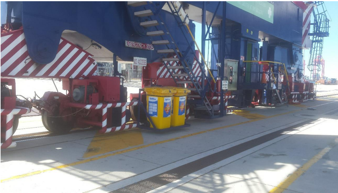
Plate 6: Spill kits conveniently located on gantry crane
