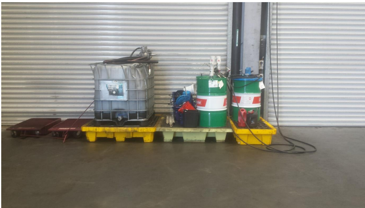
Plate 2: Spill pallet under liquid chemicals & lubricants in workshop
