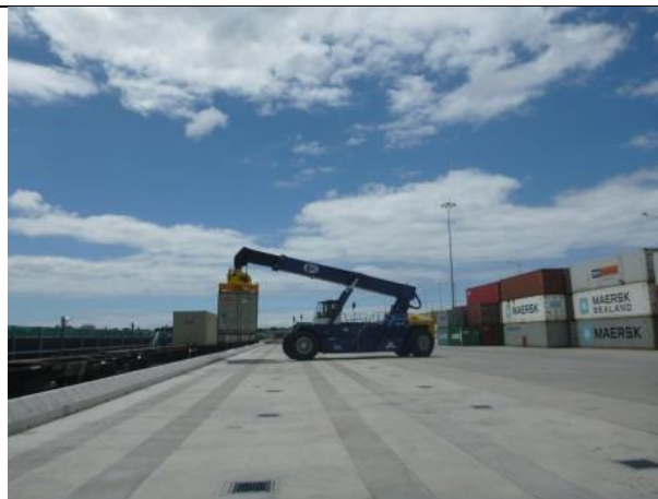
Photo 20: Spreader on reachstacker loading container onto rail wagons ✓
