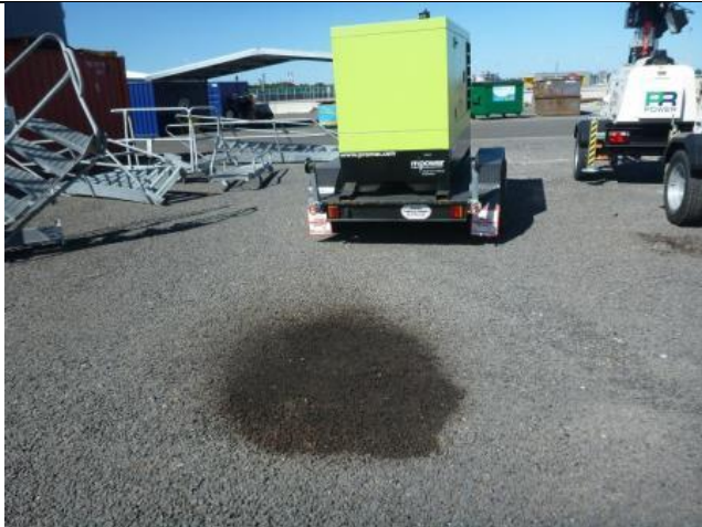
Photo 3: Evidence of oil spill on hardstand in storage area. Refer to EM IOC 3
