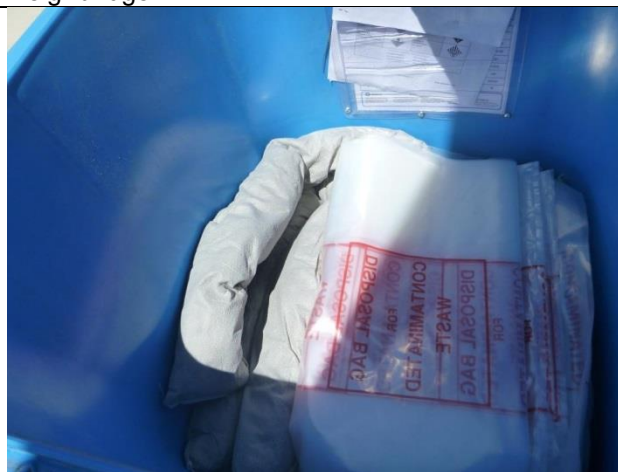
Photo 16; Inside spill kit showing organic booms and waste bags ✓
