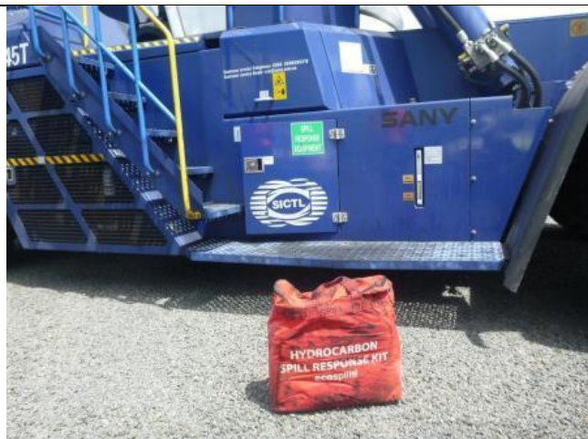
Photo 13: Hydrocarbon spill kit kept in items of plant to deal with minor spills or leaks ✓
