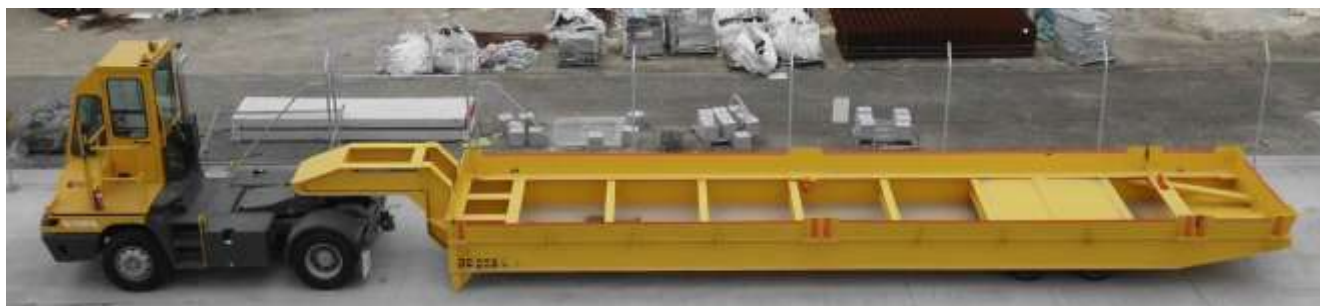
Figure 9 The bunded trailer for leaking containers upto 45' long.
