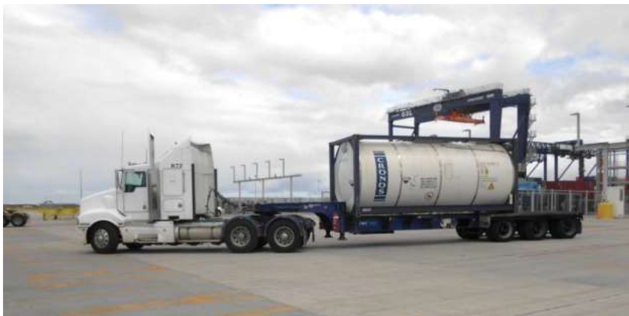
Figure 20 A 'tanktainer'/ISO tank carrying a Class 8 Dangerous Good loaded aboard a 'stepped' (low) trailer that is prescribed for this type of cargo.
