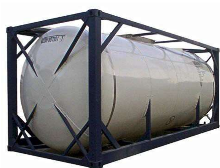
Figure 5 Example of a 'tanktainer' for the transport of liquid cargo.
